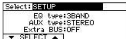
When the Extra BUS is switched ON, the BUS ON/OFF page will appear between the SETUP page and the CHANNEL ON/OFF page at the Select: field.
