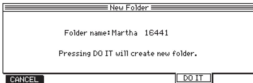
Pressing [F5] (DO IT) key, after the folder is named following the [NUMBER/NAME] key press, will create the new folder and the directory window shows the new folder being selected on its left list.
